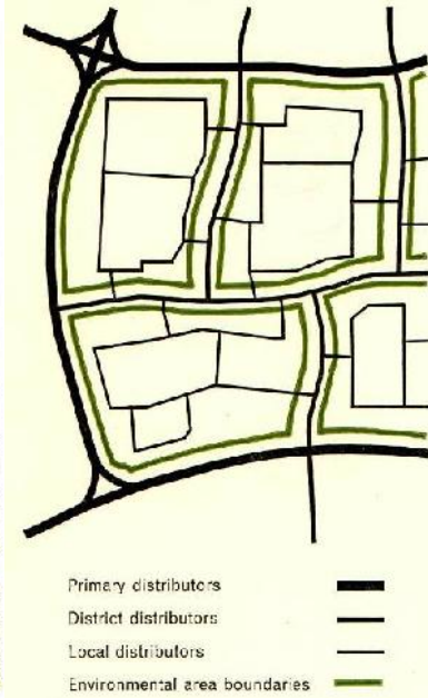
59 The principle of the hierarchy of distributors. Access roads are not shown.
