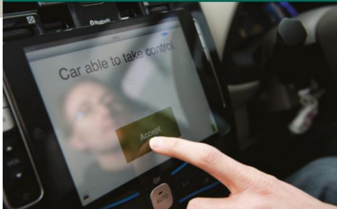
Figure 2 – The human control interface from the Oxford Mobile Robotics Group's automated Nissan Leaf vehicle
