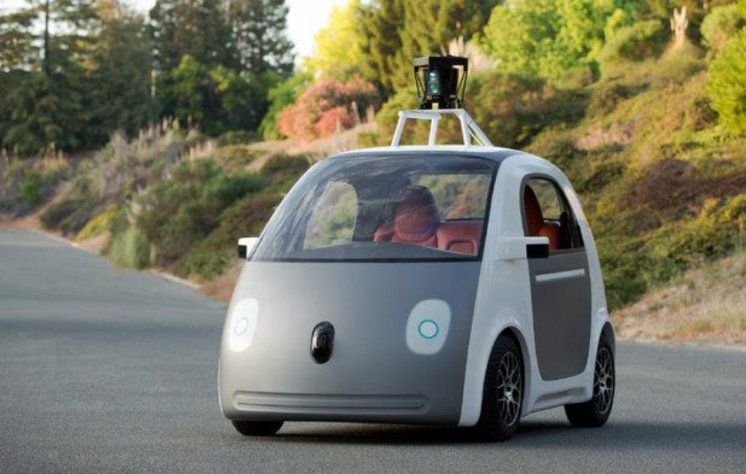
Lidar: Light detection and ranging system
