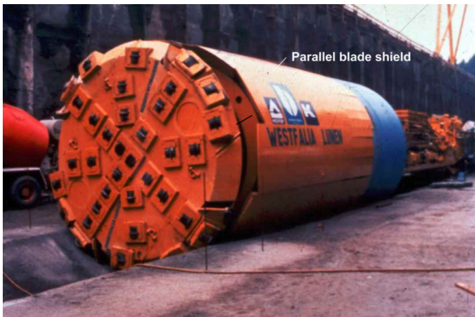
Fig. 23: Blade shield tunnel boring machine for squeezing ground conditions. The shield consists of parallel blades that are supported on hydraulic rams that can operate independently. Photograph provided by Dr Siegmund Babendererde.
