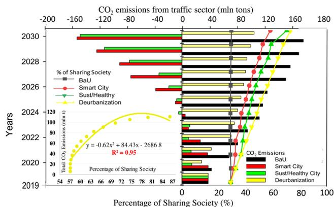
Fig. 4. Percentage of the sharing society, its impact on CO<sub>2</sub> emissions and the development of the sharing society (as a scatter and line plot on the right-hand side), simulated for the scenarios BaU, Smart City, Sustainable/Healthy City, and Deurbanisation.
