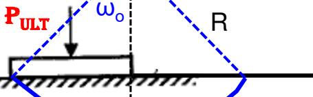
$$\tan \omega_0 = \frac{B}{h'} = \frac{12}{9} \rightarrow \omega_0 = 53.1^\circ (\hat{\omega}_0 = 0.927 \text{ rad})$$
