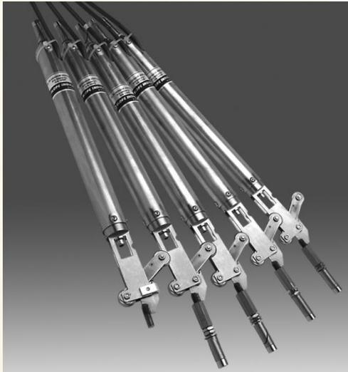
Sensors are installed with the fixed wheel pointing to the expected direction of movement.
