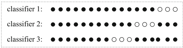
Fig. 9.1 The three classifiers were asked to classify the same 17 examples. By doing so each erred on three examples—different for each classifier. The reader can see that these errors can be eliminated by voting
