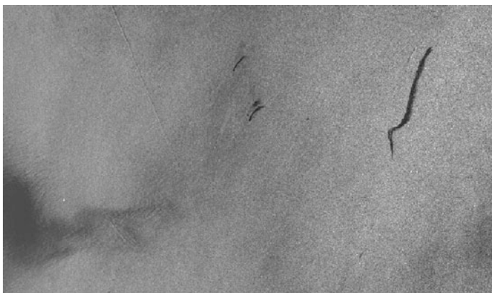
Fig. 8.2 A radar image of a sea surface. The “wiggly” elongated dark region in the upper-right corner represents environmental hazard: an oil spill
