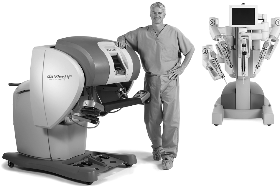
Figure 2.2 da Vinci robotic surgical system. Courtesy of Intuitive Surgical Systems.
