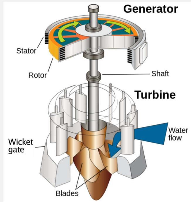
**(4)** Electro-generator (stator & rotor): **electromagnetic energy**, in the form of low-voltage alternating current (AC)
