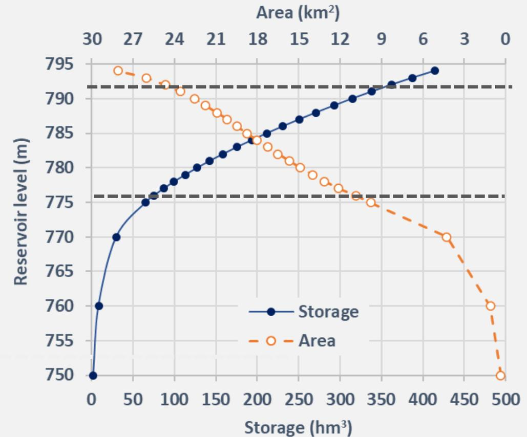
Storage-elevation-area curves for Plastiras reservoir. Minimum and maximum pool levels are +776 and +792 m, respectively, corresponding to a dead storage of 76 hm<sup>3</sup> and a total capacity of 362 hm<sup>3</sup> (useful capacity: 286 hm<sup>3</sup>)
