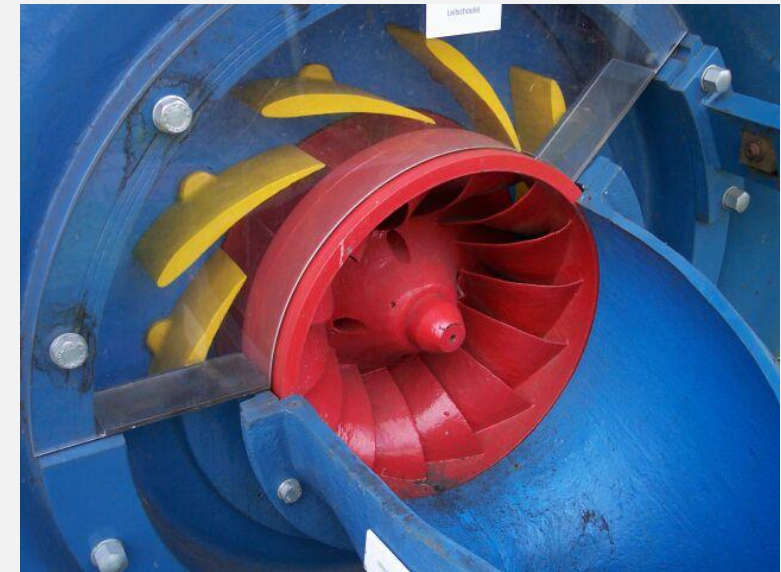
Wicket gates (yellow) at minimum (upper) and full (lower) flow settings
