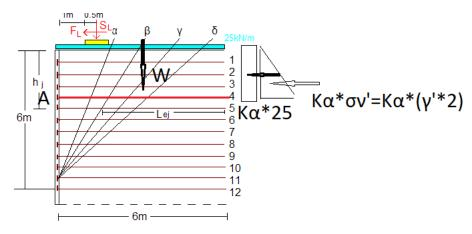
2) Lets consider the forces along reinforcement layer No4: we need  $\sigma v$  for Tpj  $\sigma v$ = 25kN/m2+4\*0.5m\*20kN/m3 +  $S_L/(6m*1m)$  simple calculation.
