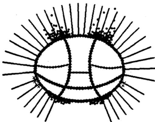
Completed excavation: yield points
