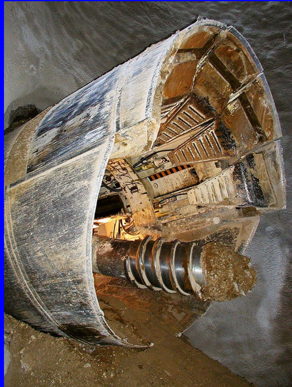
Partial Face TBM (Roadheaders)
