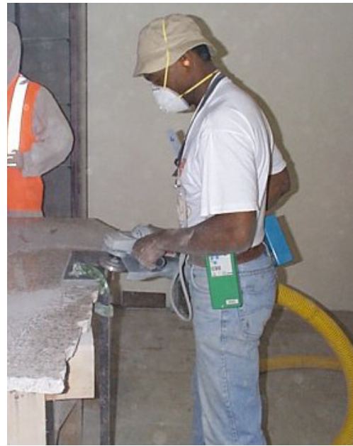
Figure 111. Example of worker wearing PPE (respiratory protective equipment and ear caps) during manual stone working
