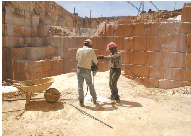
Figure 36. Vertical hole execution with a hammer
