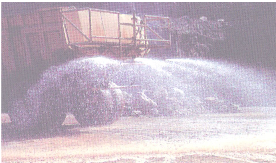
Figure 79. A water truck spraying the road in a quarry
