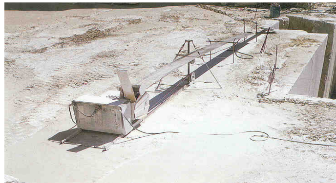
Figure 26. Diamond wire machine with safety system
