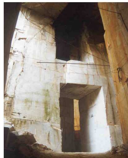
Figure 96. Pillars to support gallery vault
