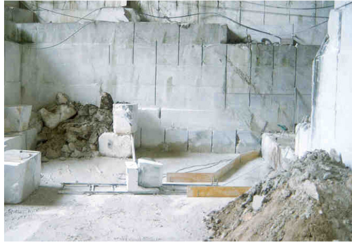
Figure 25. Horizontal cut with a diamond wire cutting machine
