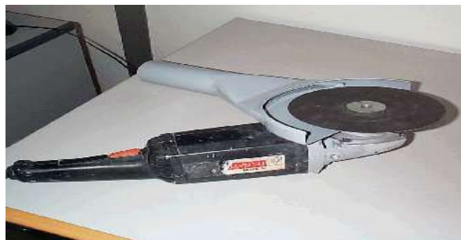
Figure 110. Dust control by a caption hood mounted on a manual tool. (ENVICUT GRD1-1999-10351 GROWTH Project report)
