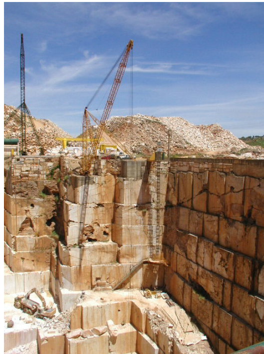
Figure 29. Lifting with derrick in a Portuguese quarry
