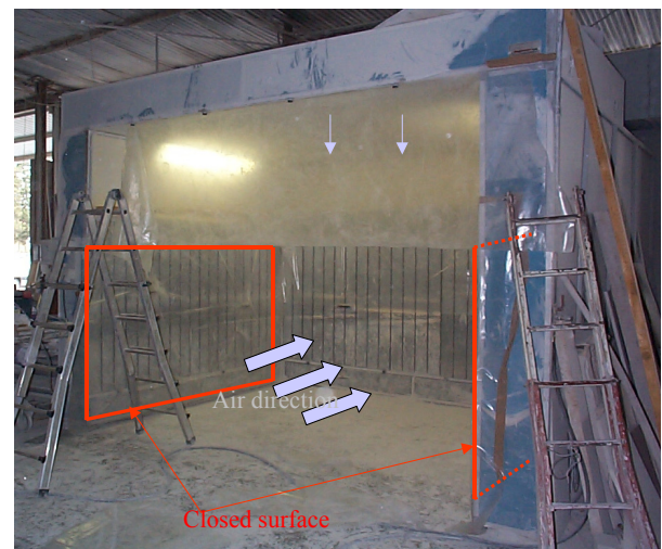
Figure 109. Dust control by an aspirating cabin. (ENVICUT GRD1-1999-10351 GROWTH Project report)
