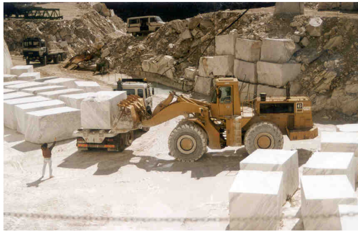
Figure 31. Block loading on truck with a power shovel
