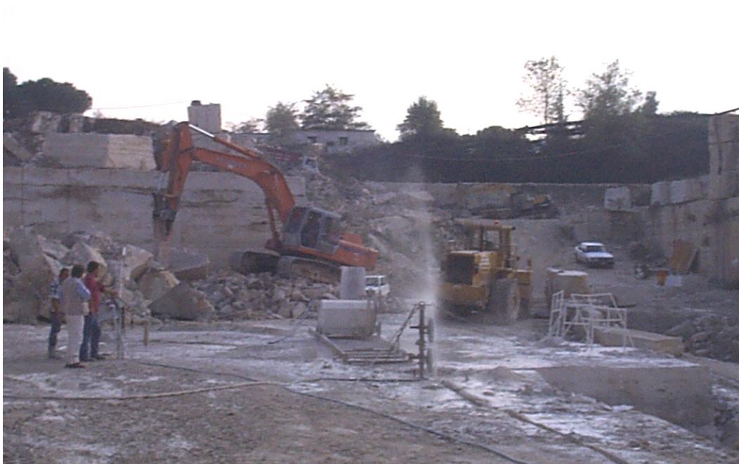
Figure 77. Sawing with a wire cutter machine
