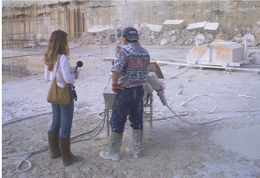
Figure 67. Monitoring of noise near a diamond wire machine
