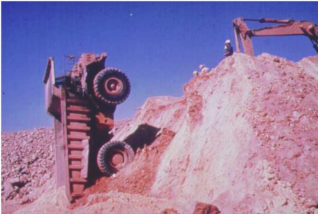
Figure 64. Example of accident in a quarry due to the lack of edge protection on roads and tips
