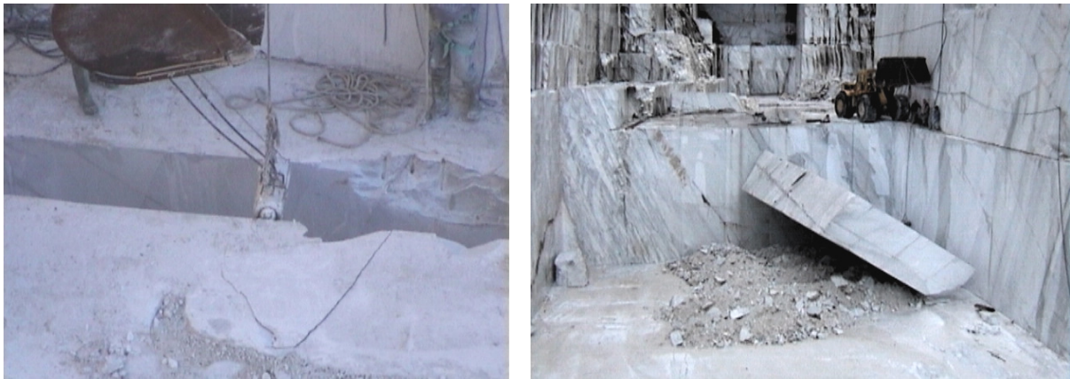
Figure 47. Bank turning over with cushion and hydraulic jack
