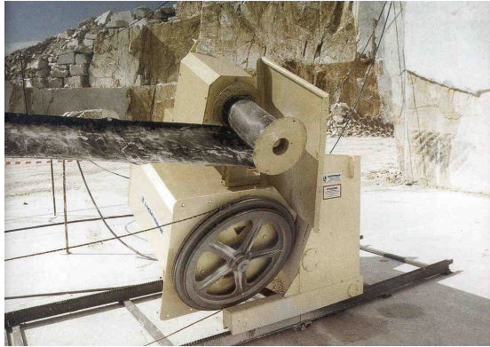
Figure 27. Diamond wire machine with a safety tape
