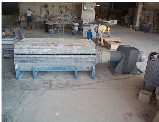
Figure 108. Dust control by an aspirating desk. (ENVICUT GRD1-1999-10351 GROWTH Project report)
