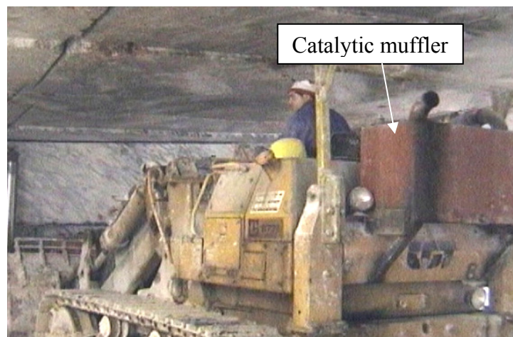
Figure 101. Exhaust gas reduction with catalytic muffler
