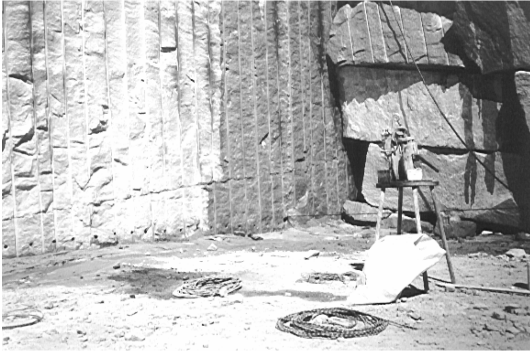
Figure 84. Block extraction (size 6x6x3 m) with explosives
