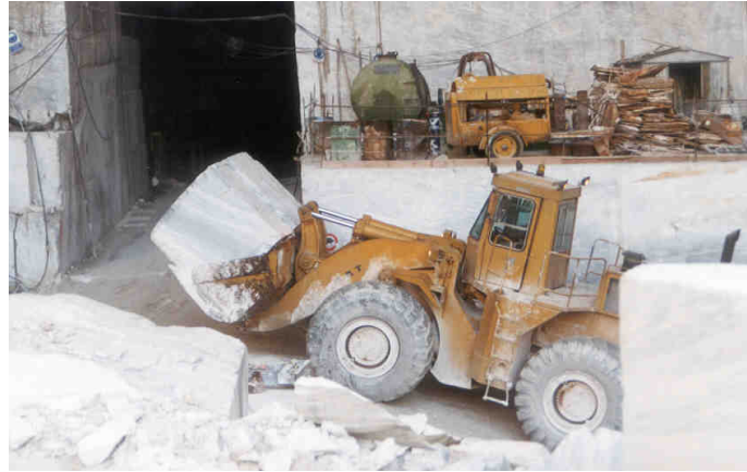
Figure 30. Block handling with a power shovel
