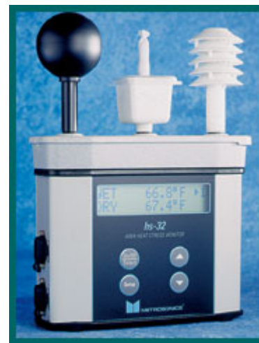
Figure 86. Example of a typical Electronic Direct-Reading WBGT Instrument (Metrosonics Inc.)
