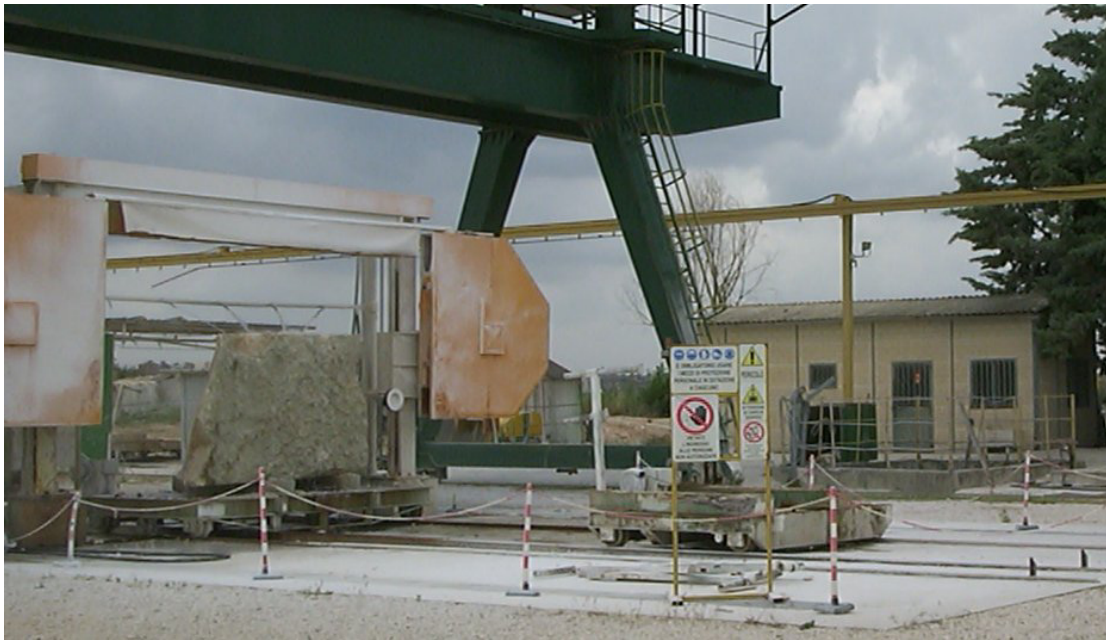
Figure 66. Example of barriers and warning signs in the area of blocks squaring
