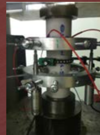
Figure 22: Testing of a cylindrical stone specimen according to the ISRM test method
