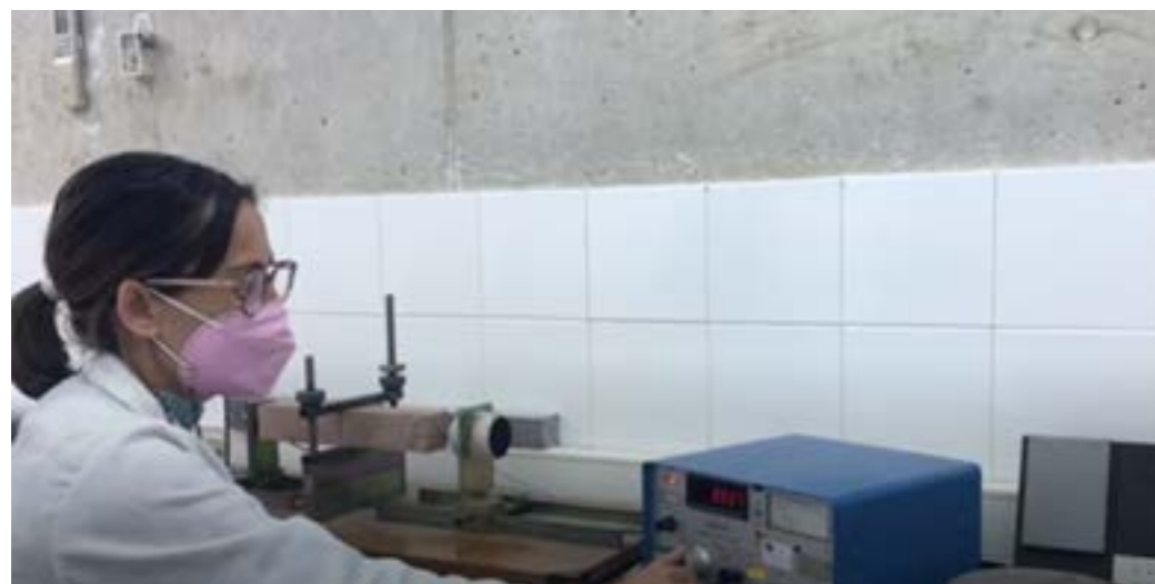
Video 8: Measurement of the frequency of the specimens. (Source: Centro Tecnológico del Mármol, Piedra y Materiales)
