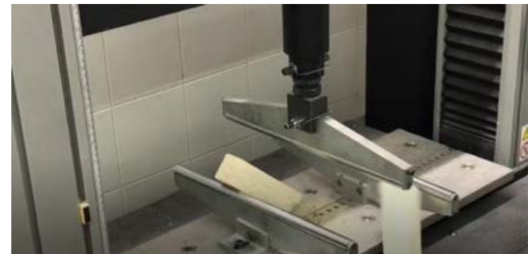
Video 7: Flexural strength under concentrated loading. (Source: Centro Tecnológico del Mármol, Piedra y Materiales)
