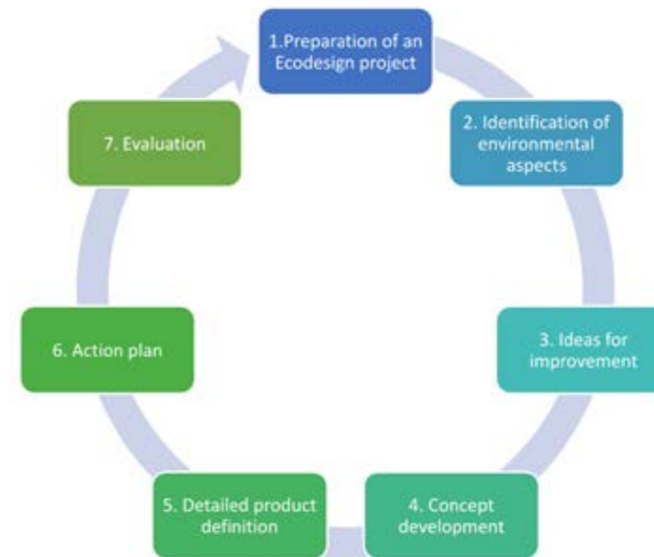
Figure 8: Development process of an Eco-design project. (Source: Centro Tecnológico del Mármol, Piedra y Materiales)
