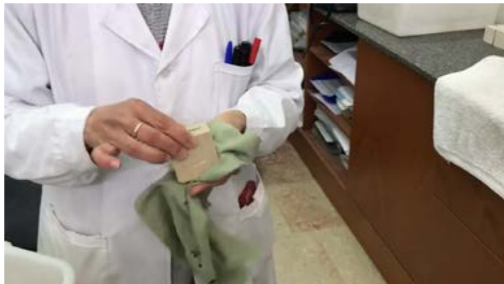
Figure 18: Removal of excess water. (Source: Centro Tecnológico del Mármol, Piedra y Materiales)
