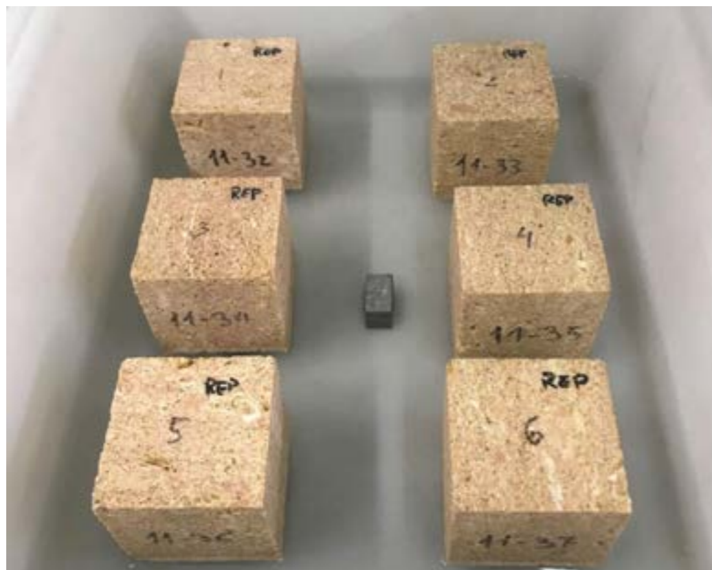
Figure 20: Specimens at the end of the test and control piece. (Source: Centro Tecnológico del Mármol, Piedra y Materiales)
