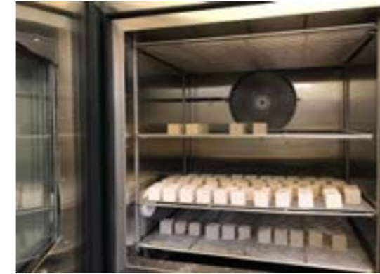
Figure 30: Wet specimens after 2 hours of immersion. (Source: Centro Tecnológico del Mármol, Piedra y Materiales)
