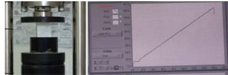
Figure 24: Testing of a cubic stone specimen according to the EN test method and continuous recording of the applied compressive load.
