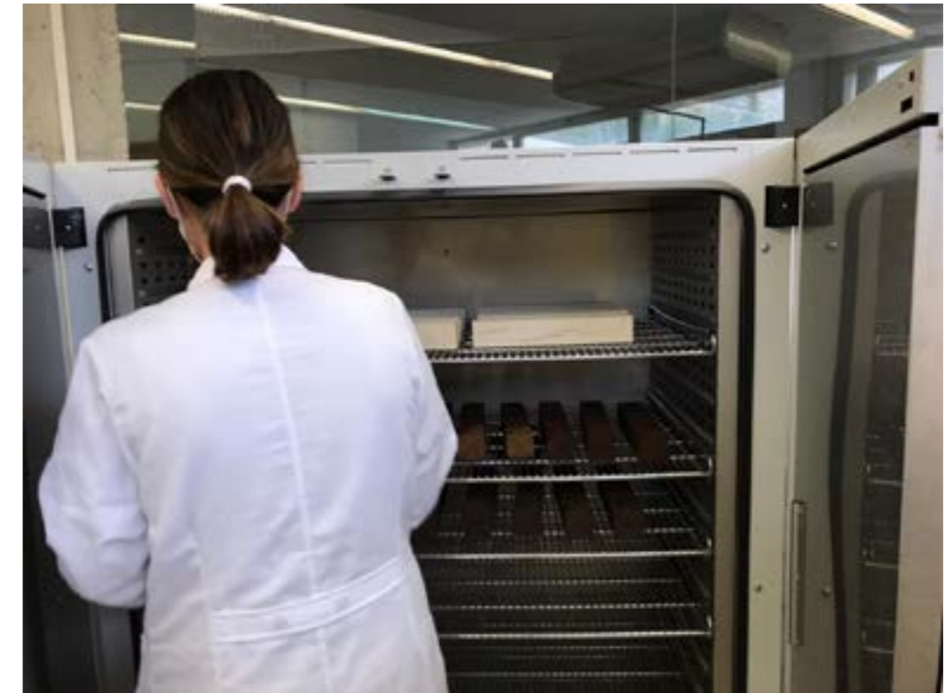
Figure 32: Introduction of the specimens into the oven. (Source: Centro Tecnológico del Mármol, Piedra y Materiales)
