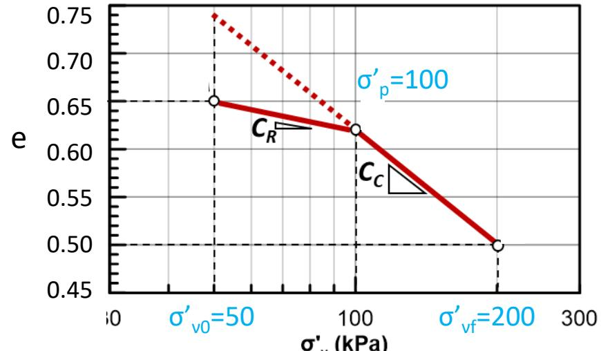
$$\rho = \frac{H}{1 + e_o} \left[ c_r \cdot \log \frac{\sigma'_p}{\sigma'_{v,0}} + c_c \cdot \log \frac{\sigma'_{vf}}{\sigma'_p} \right] = \frac{10}{1 + 0.65} \left[ 0.05 \cdot \log \frac{100}{50} + 0.25 \cdot \log \frac{200}{100} \right] = 0.55m$$
