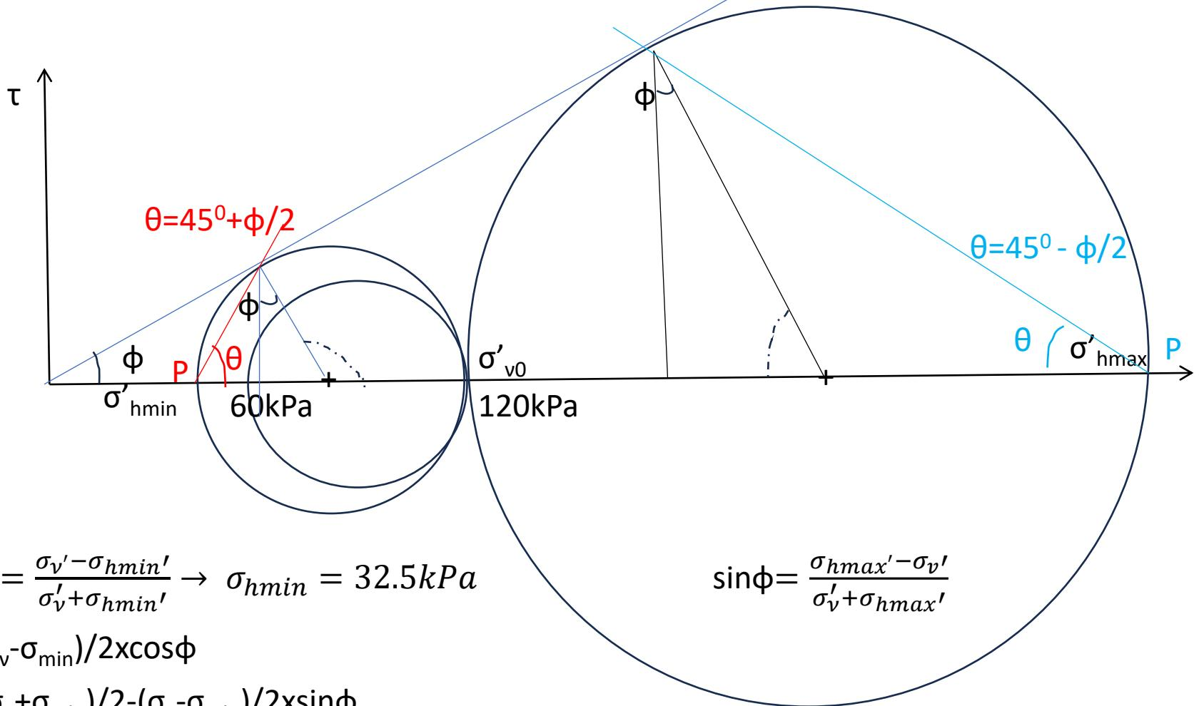
$$\sin\phi = \frac{\sigma_v' - \sigma_{hmin}'}{\sigma_v' + \sigma_{hmin}'} \rightarrow \sigma_{hmin}' = 32.5 \text{ kPa}$$
