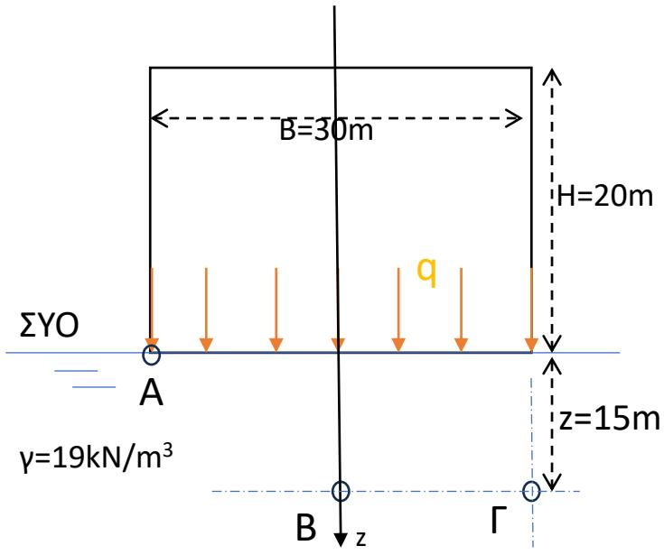
$$q = 7.5 \text{ kN/m}^3 \times 20 \text{ m} = 150 \text{ kN/m}^2 (\text{kPa})$$
