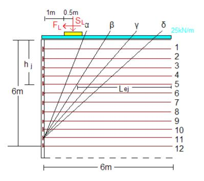
Please note: the water table lies beneath formation level; omit factors of safety to loads and soil parameters to facilitate calculations; tabulate calculations; use ReActive to define critical failure mechanism and required  $T_{max}$ .
