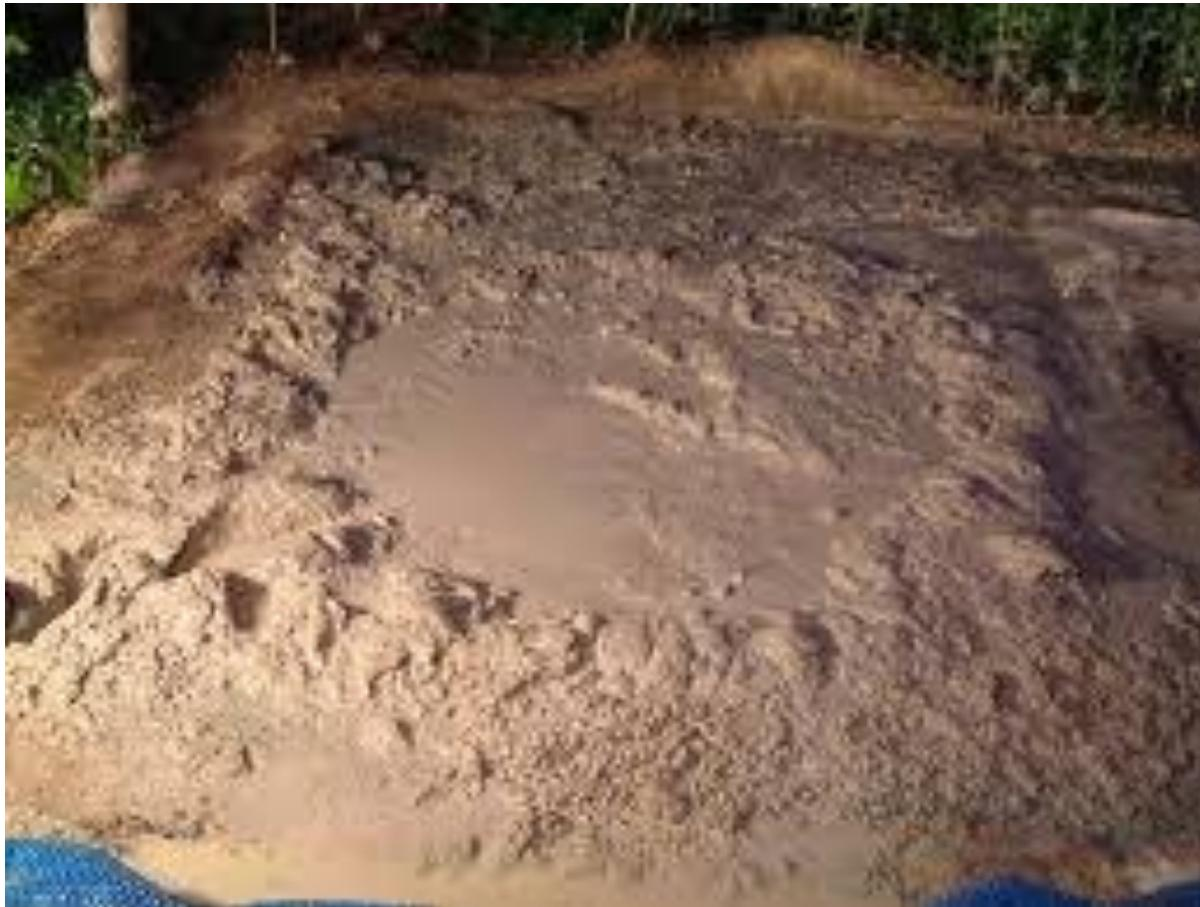
1. Sand has no strength due to LIQUEFACTION or due to SOIL PIPING
