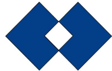
A XOR B (A + B) - (A X B) A or B, but NOT both
