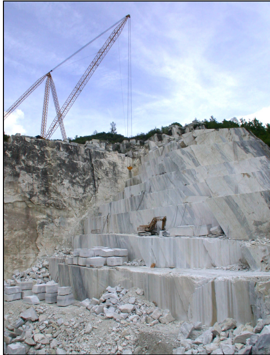
Figure 51. Derrick crane in a hillside marble quarry (Italy).
