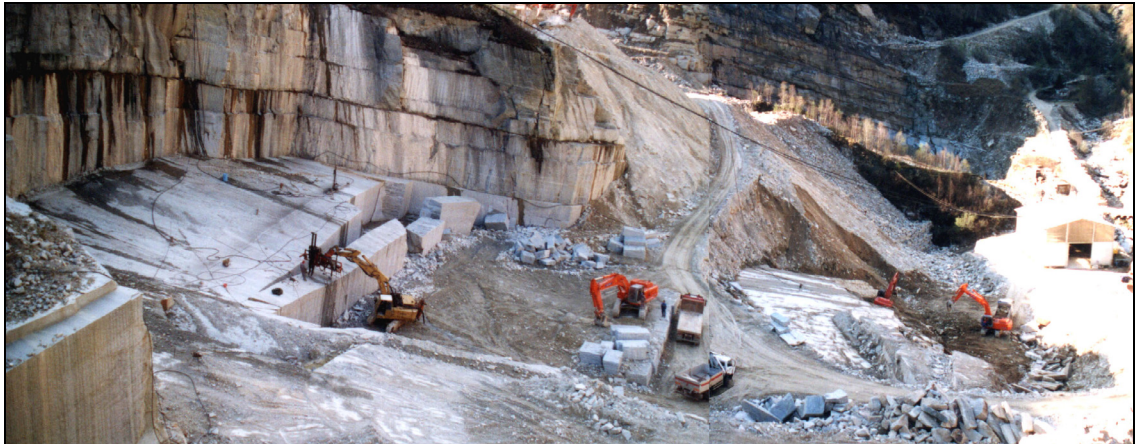
Figure 46. A typical alpine quarry of gneiss, exploited through dynamic splitting technology.
