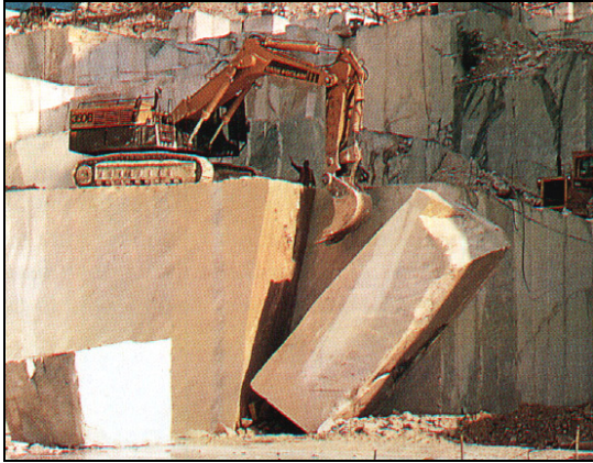
Figure 42. Marble quarry: overturning a high bench, cut with diamond wire.
