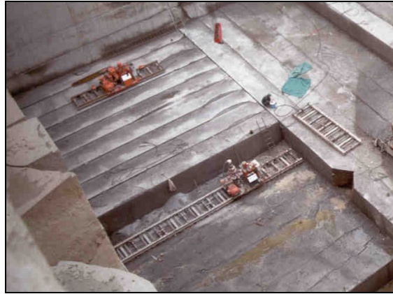
Figure 43. Tuff quarry exploited only by chain cutters (Italy).
