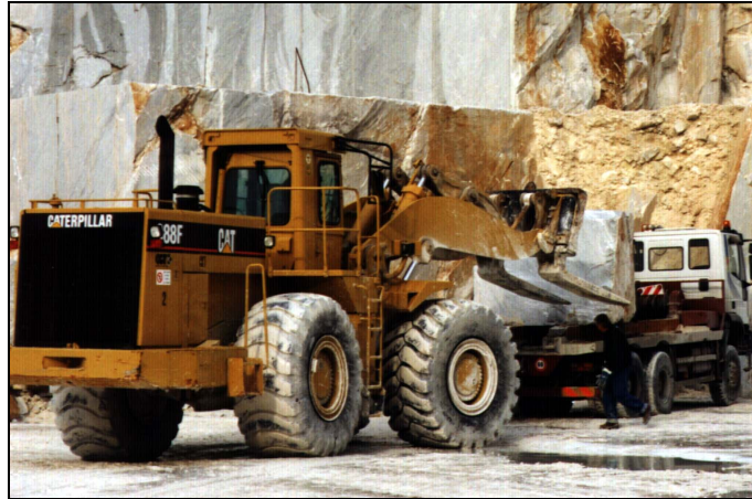
Figure 50. Wheeled loader equipped with “fork” for loading of marble blocks on truck.
