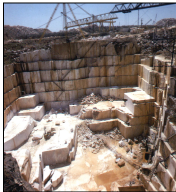
Figure 30. Quarry of calcareous stone in flat land with very deep pit layout, exploited in many levels (Italy).
