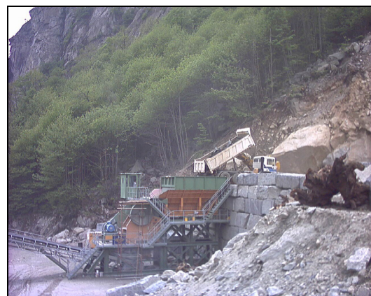
Figure 67. The installation of a mobile or fix crusher in a area next to the quarry can reduce the costs of transport of the material and realize an integral reuse of the quarry waste.
