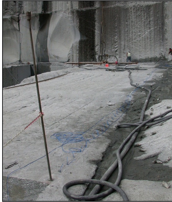
Figure 23. Splitting by explosive of a great bank of gneiss (Val d' Ossola - Italy).
