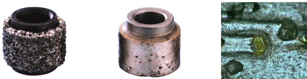
Figure 12. From left: an electroplated bead; one sintered; a microscope magnification of diamonds at the surface of a sintered bead.
