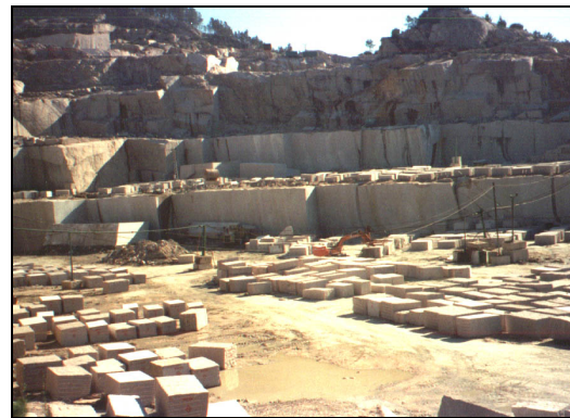
Figure 31. Flat land quarry of pink granite, with stepped layout (Spain).
