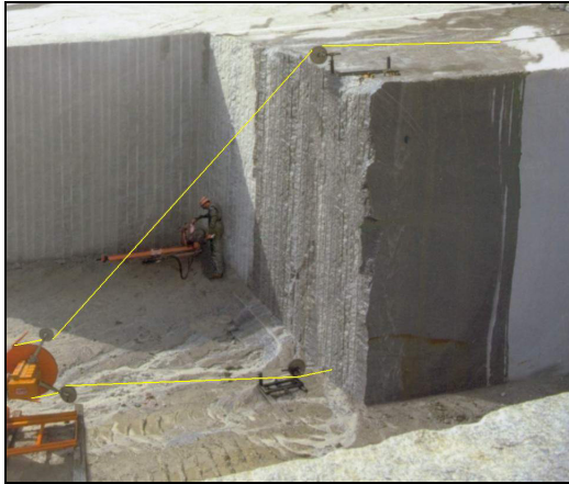
Figure 9. Cutting by diamond wire with traditional “descending loop”.
