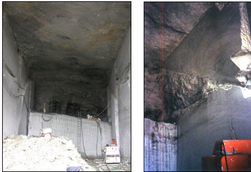
Figure 57. The tunnel-quarry in the first productive phases. On the right, a detail of the cut of the upper wedge.
