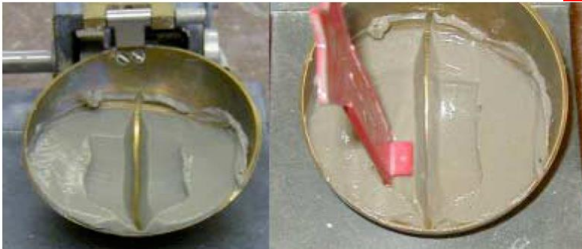
Figure 3 - Left, groove separating two halves of pat, right, stop blow counts after this length of groove closes a length of 13 cm.
