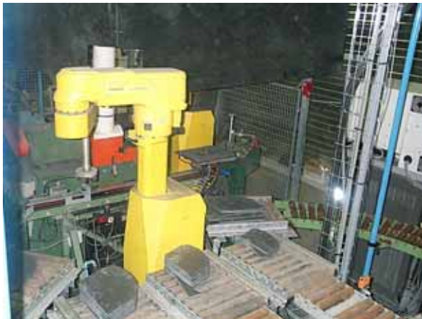
Figure 87. Final production phase: sorting the slates and rejecting the defective ones (at the far right hand side).
