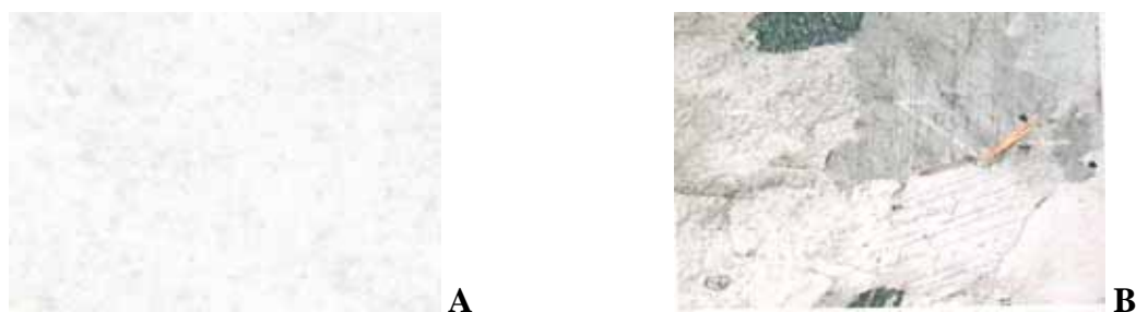
Figure 53. Calcite marble (Greek). A: macroscopic image of the hand specimen, B: microscopic image of a thin section in crossed polarised light
