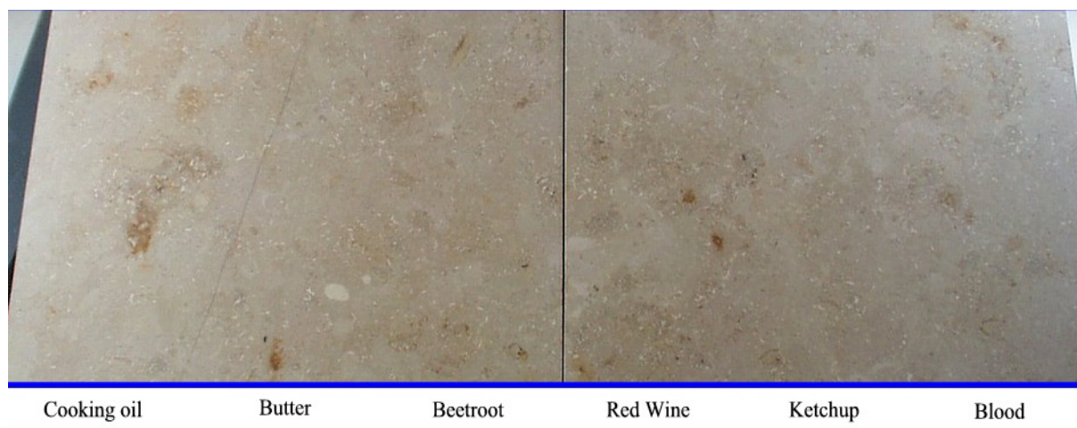
Figure 134. Picture of stain test. Limestone with surface impregnated by perm-coat
