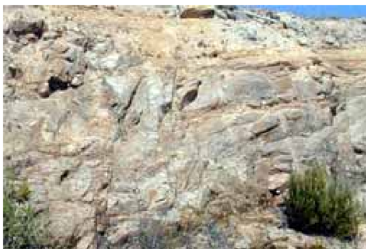
Figure 27. Effects of weathering on a granite outcrop; the decay in the physical properties of both the rock massif and the intact rock is visually perceptible.
