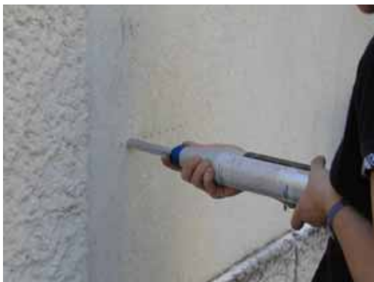
Figure 79. Type L Schmidt hammer for in situ testing of a stone cladding.
