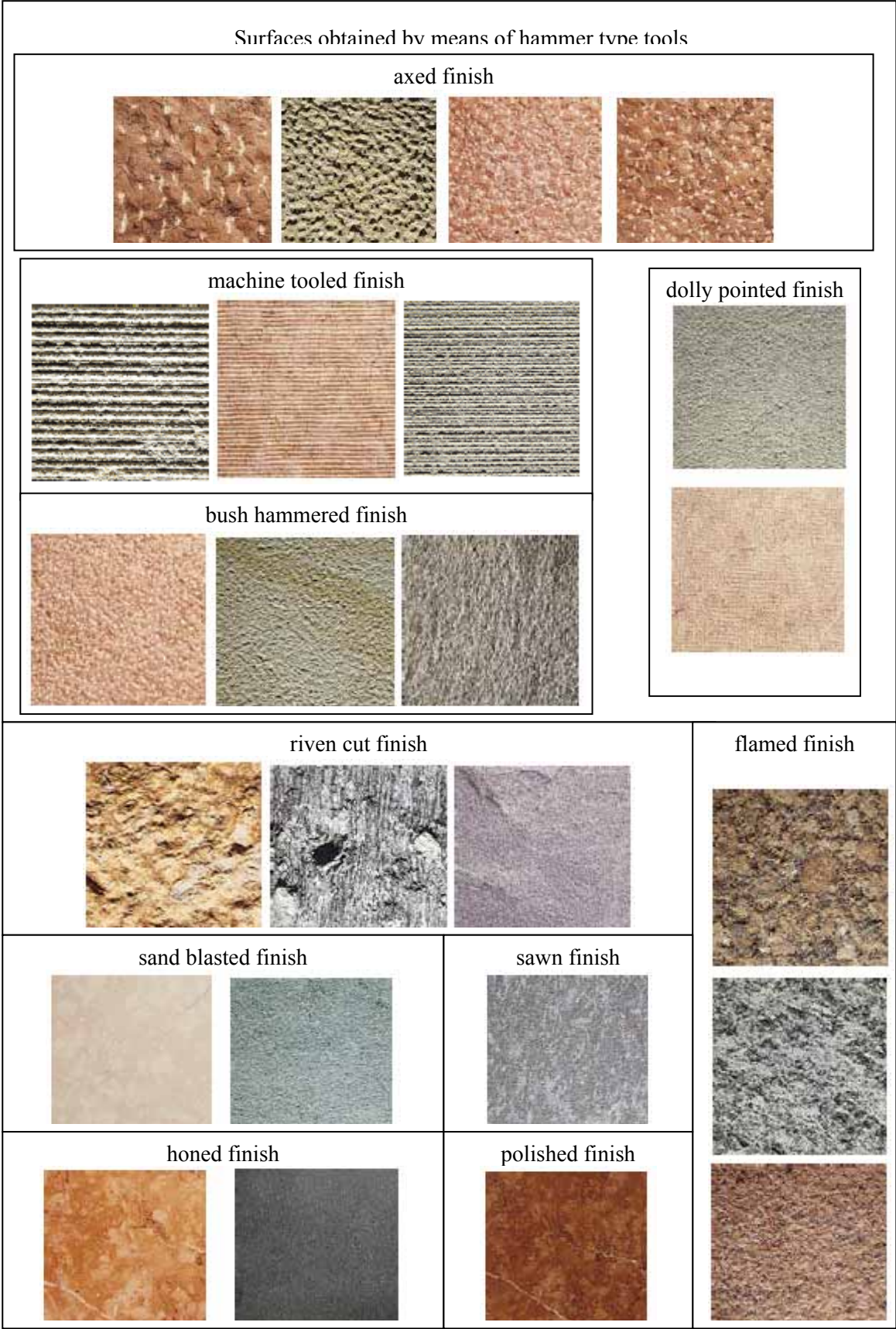
Figure 46. Examples of surface finishes.
