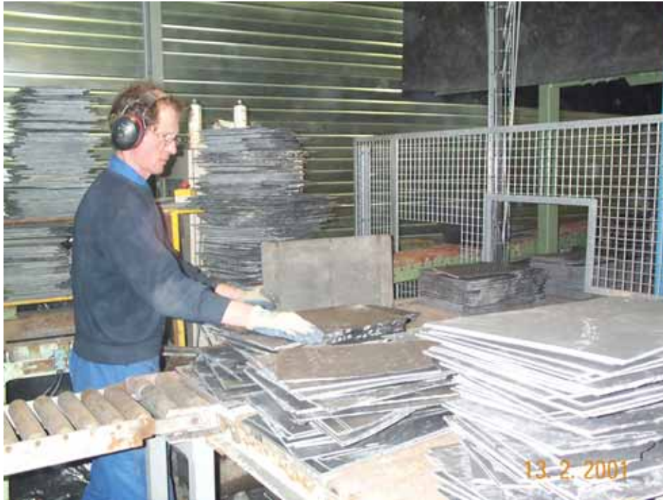
Figure 86. The only slate worker between the splitting machine and the production line incorporating the artificial vision and vibratory analysis methods.
