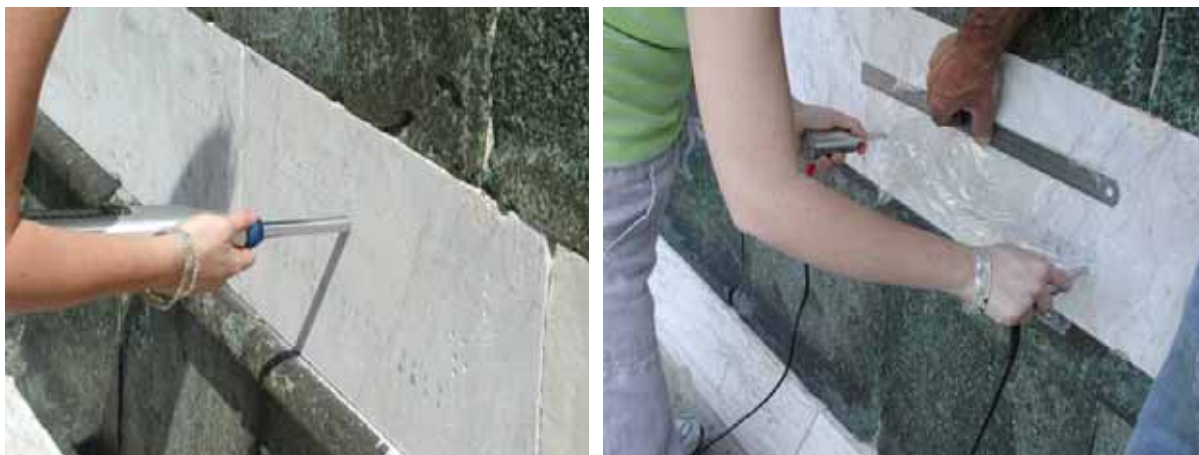
Figure 146. Testing deterioration of internal structure and hence the strength. To the left a Schlerometer and to the right Ultrasonic velocity test
