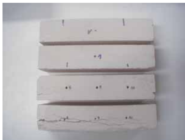
Figure 129. increasing damages on specimens of the same type of stone after the same number of freeze-thaw cycles but with increasing impregnation rates
