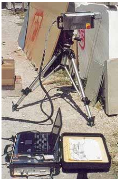
Figure 78. Measurement of the drilling resistance by means of the DRMS device on a marble block.
