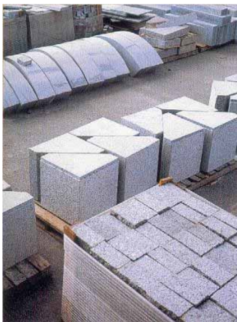
Figure 50. Transport-ready pieces of dimensional stones.
