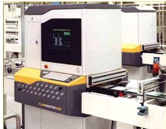
Figure 99. Industrial plant image selection system (Surface Inspection – Flow Master).
