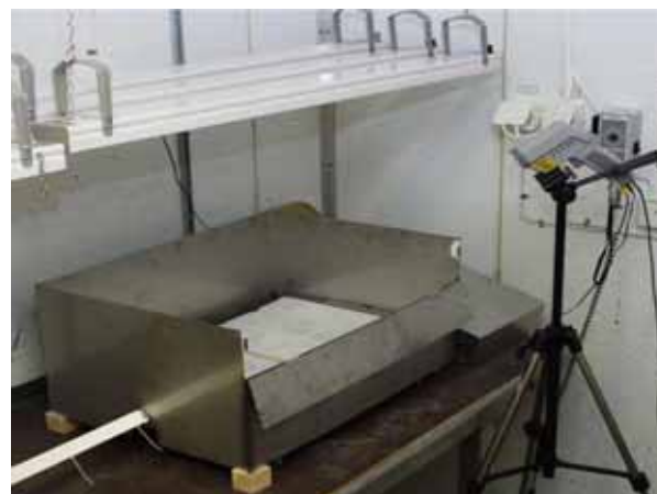
Figure 145. Laboratory testing for the bowing potential of marble (NORDTEST, draft method)
