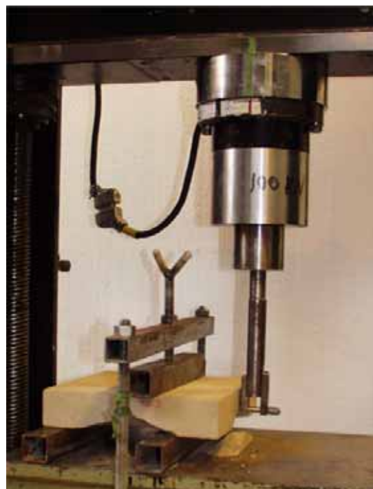
Figure 131. Test rig for break load at dowel hole
