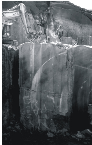
Figure 16. Slicing a loose primary block. "Labrador Antique" quarry, SW Norway.
