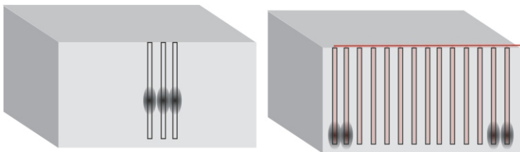
Figure 21. Two examples of granite splitting with the use of explosives. Left: black powder (dark spots) in three central holes placed along the primary cleavage plane of the granite. Right: detonating fuse (red line). In this example, combined with black powder only in the marginal holes
