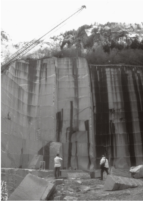
Figure 33. Steep hillside quarry, "Serizzo"-gneiss, Northern Italy.
