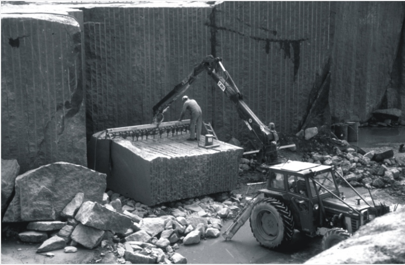
Figure 26. Hydraulic wedging in a larvikite quarry, Norway.
