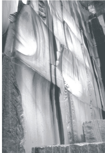
Figure 19. Curved surface after wire sawing in serizzo (gneiss)-quarry, Northern Italy. The curving is due to stress.
