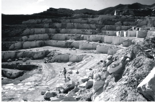
Figure 31. “Theatre-shaped”, well planned marble quarry, Athens, Greece.
