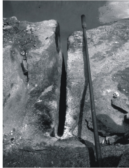
Figure 27. Channel from jet-burning in granite quarry and jet-burner (right).
