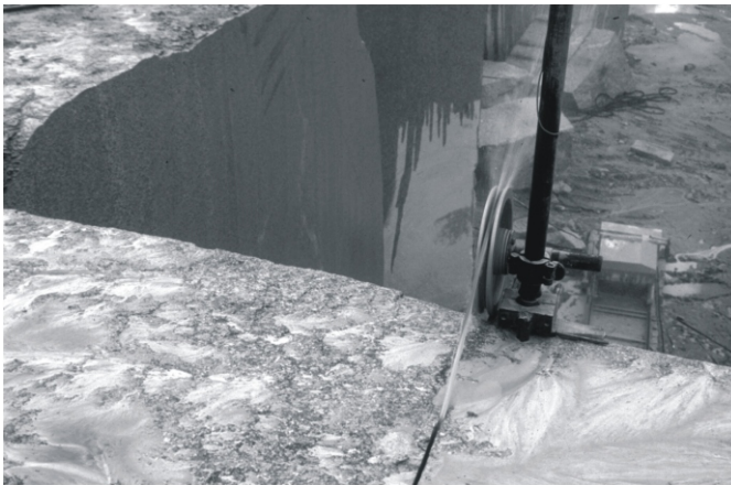
Figure 18. Diamond wire sawing in a granite quarry, Spain
