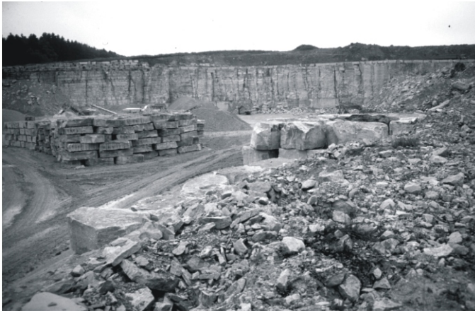
Figure 39. Only the lowermost part of this limestone formation in Germany is usable for ornamental stone. The rest is applied for aggregate and cement.
