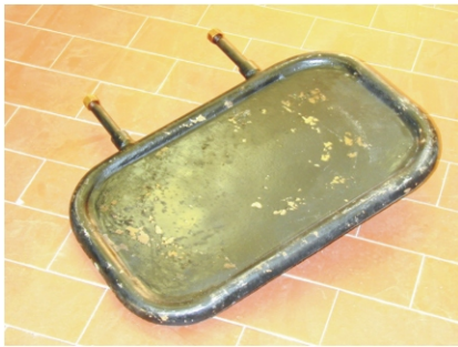
Figure 46. a) flat pressure cell for the measurement of the natural stresses by restoration of the stresses; b) scheme of the measurement displaying the cut executed in order to position the pressure cell and the measure bench marks (Fritz & Kovari, 1999).
