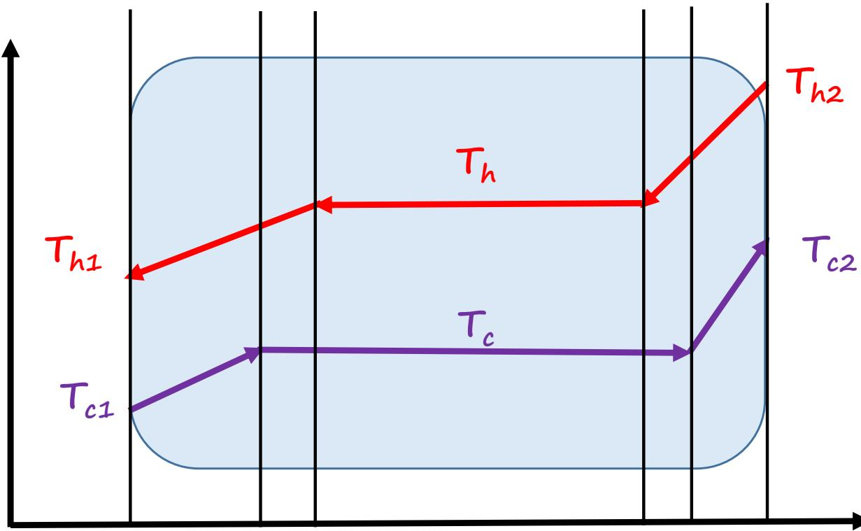
$$Q = F_h C_{PhL} (T_h - T_{h1}) + F_h \Delta H_h + F_h C_{PhV} (T_{h2} - T_h)$$
