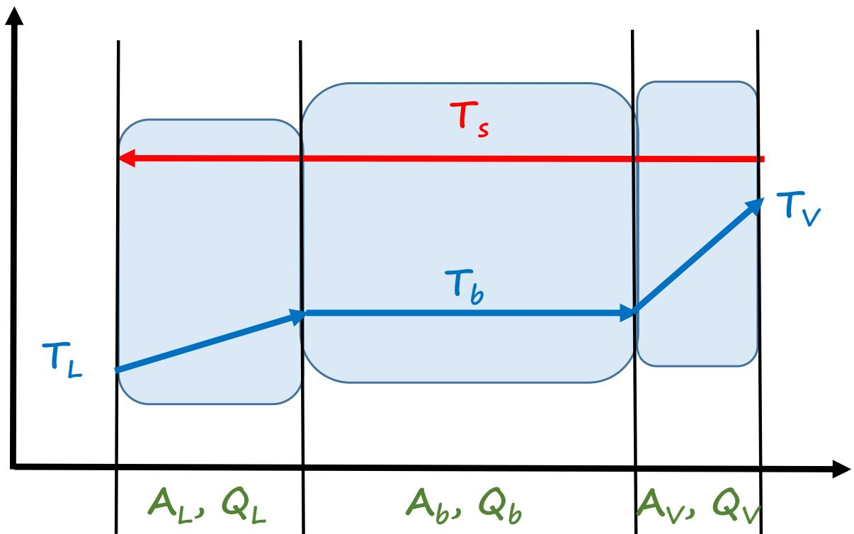
$$Q_L = A_L U_L \Delta T_L (T_s - T_1, T_s - T_b)$$
