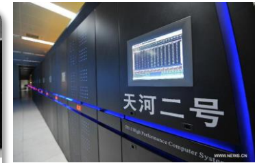
2015 Tianhe-2 (MilkyWay-2): Intel Xeon E5-2692 12C 2.200GHz, Intel Xeon Phi ti1S1P, ti.12M cores, 1,024 TB RAM, 50 PFlops, 17,8 MW
