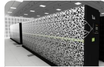
2012 Bull B510, 10K cores, 4TeraBytes RAM, 200 TFlops
