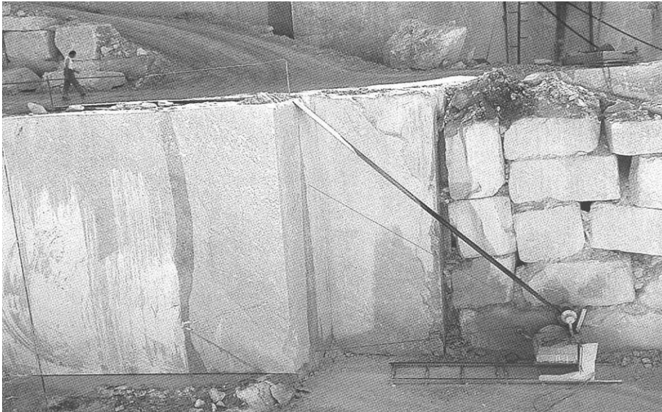
Figure 9. Diamond-wire saw, source: Frederick Bradley, Marble Quarrying/Technical and Commercial Manual , 1999
