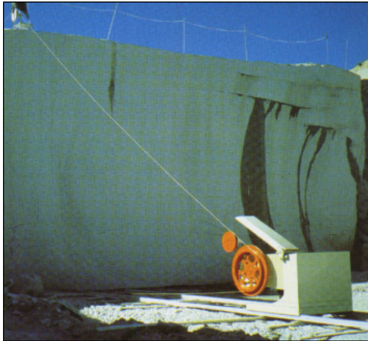
Figure 76. Diamond wire in the quarry
