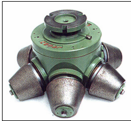
Figure 121. Rotary calibrating heads (with conical tools)
