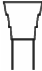
Figure 88. Section of a “Pagoda” Segment
