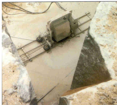
Figure 2. Primary cut with diamond wire
