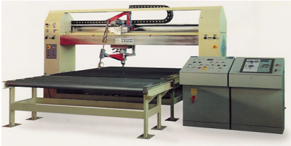
Figure 61. Flaming machine for slabs
