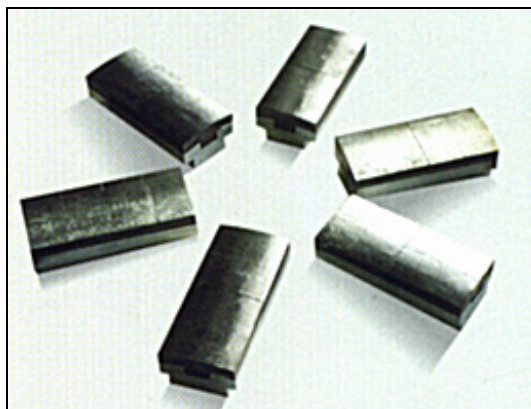
Figure 132. Diamond polishing tools for Polishing heads with oscillating arms (granite)
