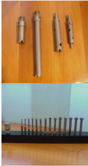
Figure 156. Diamond drill cores and diamond drill bits
