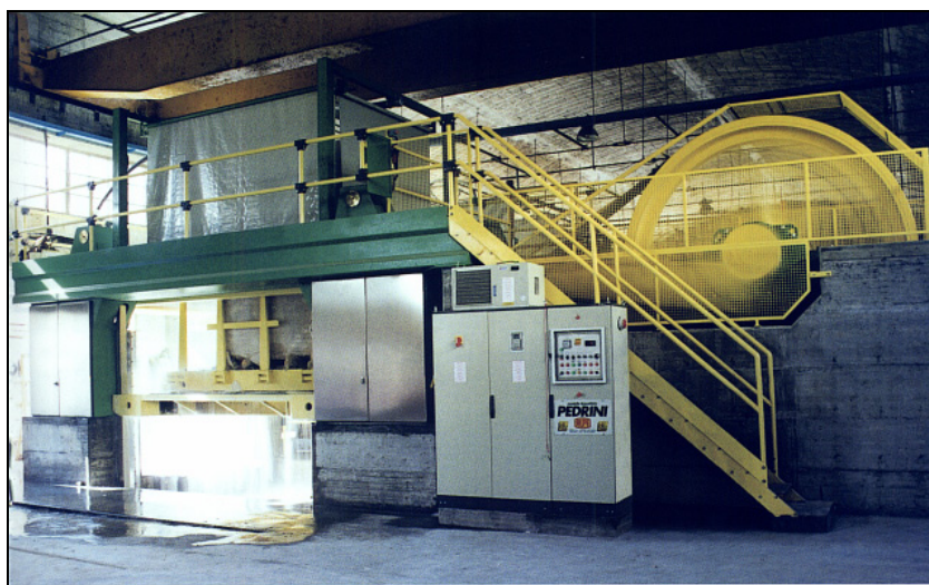
Figure 25. View of an 80 blades diamond frame for marble
