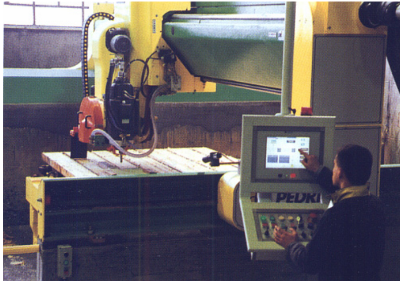
Figure 63. A modern CN bridge milling machine in operation
