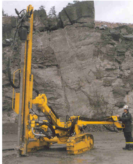
Figure 13. View of down-to-hole hammer
