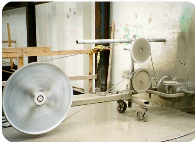
Figure 1. View of diamond wire cutter (Concrete)
