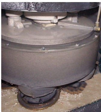
Figure 122. Rotary calibrating head (with conical inclined satellite tools)
