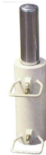
Figure 180. View of hydraulic jacks
