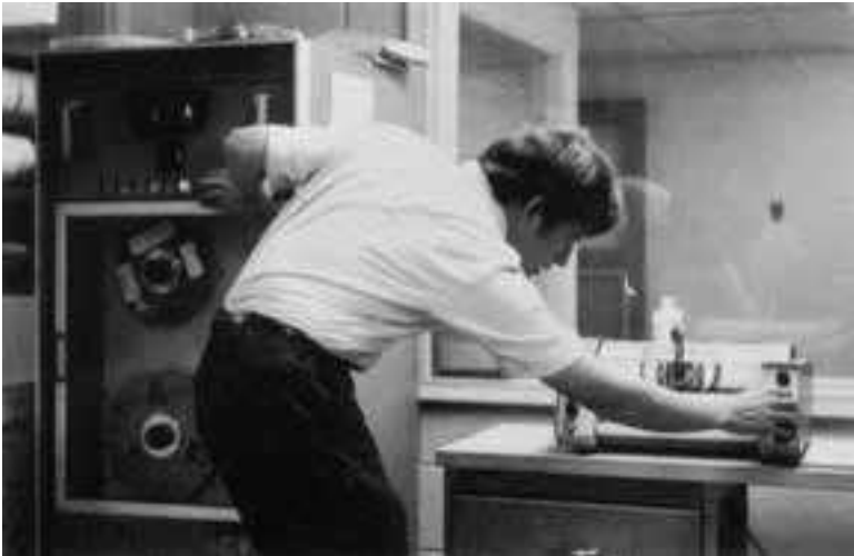
FIGURE 3.1 Lloyd Sumner generating computer art with a Burroughs B5500 computer and Calcomp 565 plotter, ca. 1968. University of Virginia. Courtesy of Jean Sumner.
