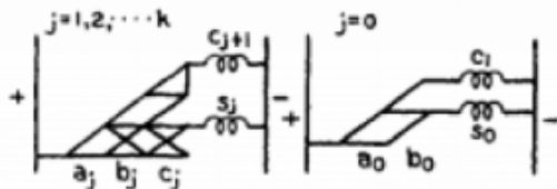
Figure 35. Circuits for electric adder
